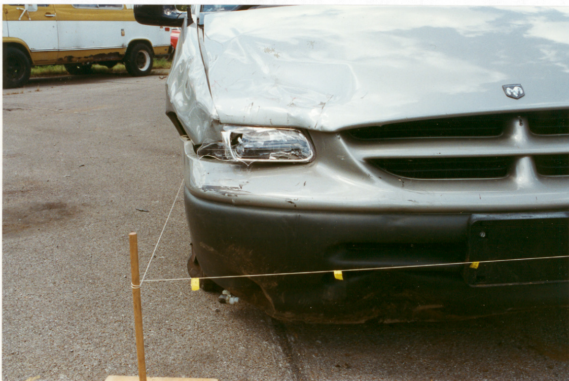
30. View of the direct contact damage to the Dodge Caravan.
